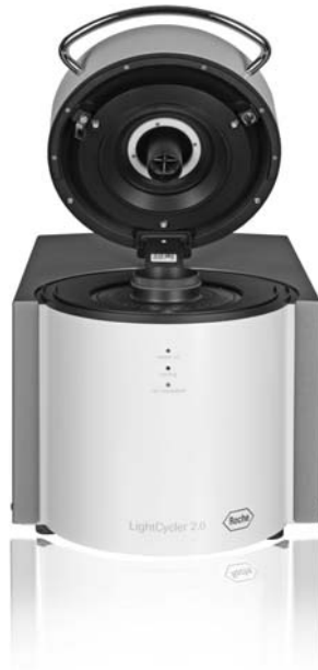
Figure 19.2 LightCycler® 2.0 real-time PCR system shown with the top open. The instrument holds up to 32 samples in specially designed glass capillaries that travel on a rotating carousel during the PCR process. Courtesy of Roche Applied Science.
