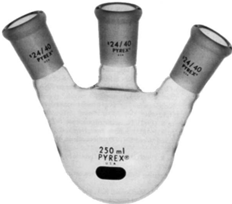
Figure 7.2 The three-neck flask configuration permits easy access to the reaction components and mounting of a pH electrode, thermometer, and N 2 stream. Photograph courtesy of Corning Glass, Corning, New York.
