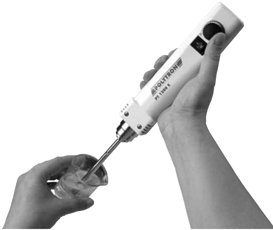
Figure 3.1 Polytron ® homogenizer. Models range from hand-held units (shown) to dispersing machines with throughput capacity up to 130,000 L/h. Courtesy of Kinematica, Inc.
