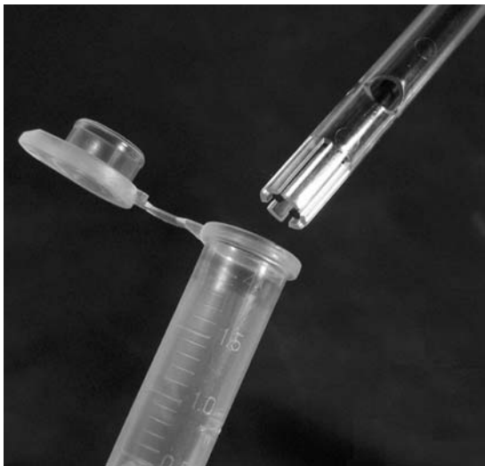
Figure 3.2 Hand-held motorized homogenizer showing disposable generator tips. Tips are simply discarded after use, minimizing the down-time required to clean generator between each sample. If desired, the tips can be cleaned and reused a limited number of times. Courtesy of Omni International.
