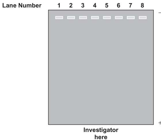
Figure 9.4 Standard nomenclature for referencing wells on a gel. The side of the gel with the wells is furthest away from the investigator who is standing in front of the gel, ready to load the samples. The wells are numbered consecutively, from left to right.
