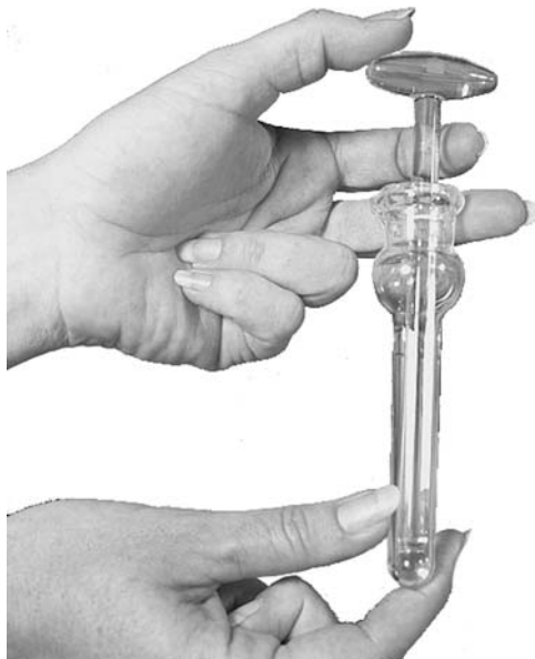
Figure 3.3 Dounce homogenizer. This handheld instrument is an effective homogenization device for many types of tissue. See text for details. Courtesy of Bellco Glass Company.
