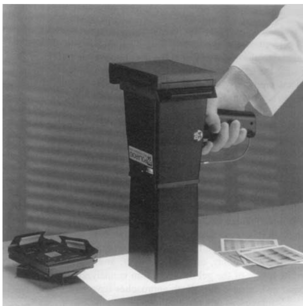
Figure 10.6 Polaroid DS-34 handheld camera. Snap-on hoods allow photodocumentation of a variety of gel sizes and they also position the camera for sharp focus. A built-in lens ensures proper magnification and focal length. Courtesy of Polaroid.
