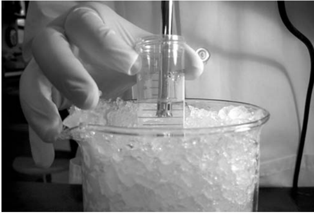
Figure 3.6 Homogenization of tissue using the LiCl-urea method. The conical 50 ml tube containing the tissue sample and the LiCl-urea homogenization buffer is held in an ice bath during the homogenization process. This is an excellent way to avoid generating heat caused by the action of the homogenizer. Short bursts of homogenization are applied, totaling no more than 60s, as described in the text. The tube is maintained in the ice bath between applications of the homogenizer.
