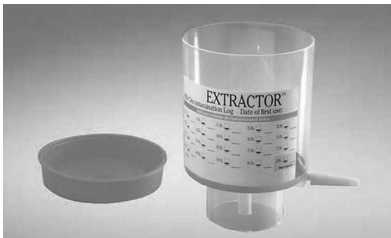
Figure E.1 Extractor filtration device for the removal of ethidium bromide and SYBR Green from electrophoresis- and staining buffers. Photograph courtesy of Whatman, Inc..
