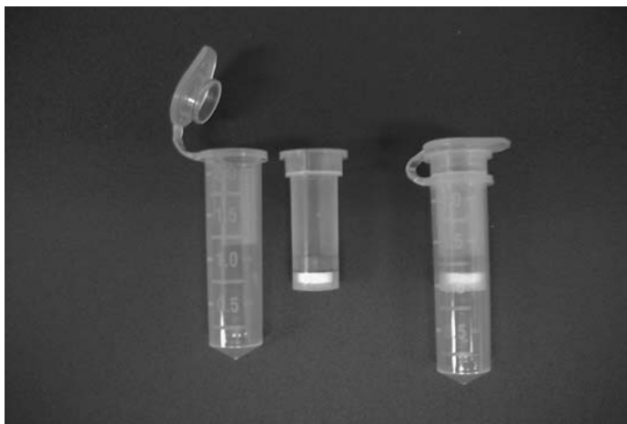
Figure 2.8 Silica filter for nucleic acid isolation. Under chaotropic, high-salt conditions, nucleic acids bind to the silica insert, while lysis buffer components and other cellular macromolecules are washed away. The purified sample is then eluted under low-salt conditions. The most commonly used filter format used in the laboratory is small enough to fit into a standard 1.7 ml microcentrifuge tube (2.2 ml microcentrifuge tube shown). Courtesy of Sigma-Aldrich.
