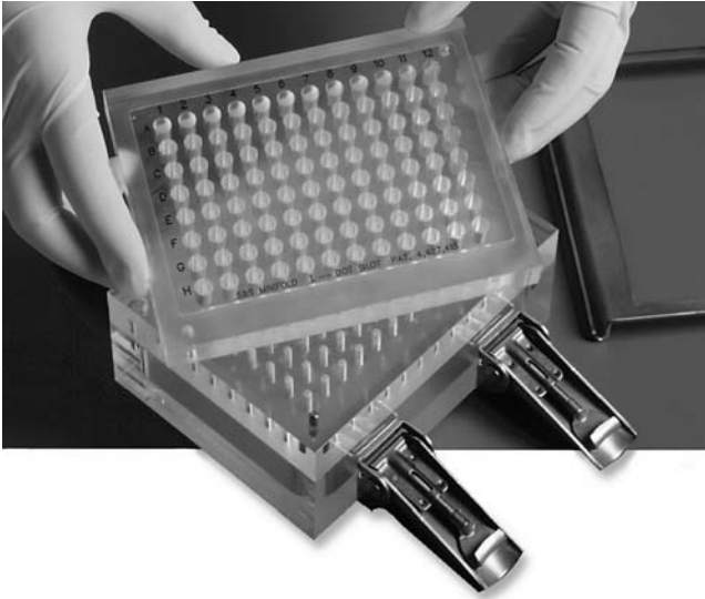
Figure N.1 Minifold® I dot blot apparatus. Sample dilutions are applied under vacuum directly to the surface of the filter membrane. Depending on the format, the sample is concentrated into either 12.5 mm 2 “dots” or 2 mm 2 “spots”. Courtesy of Schleicher and Schuell Bioscience.
